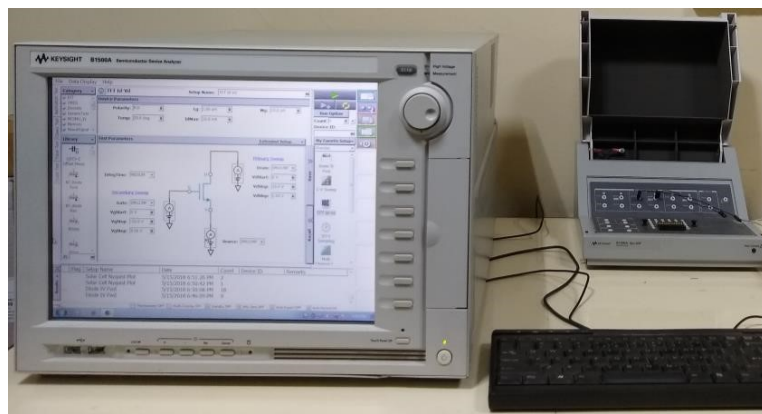
Figure 1.13: Semiconductor parameter analyser for the measurement of various electrical parameters.
