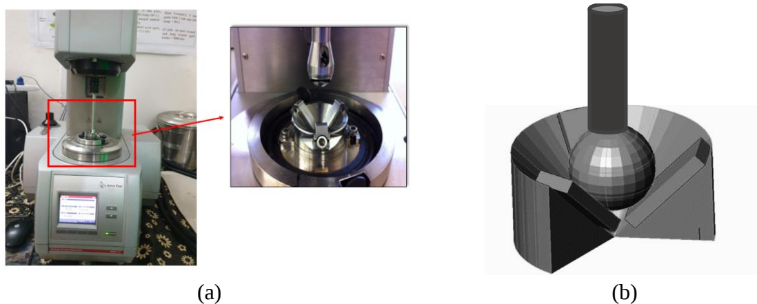
Figure 3-19. a) Ball-on-three plates arrangement mounted on DSR b) Schematic of the ball-on-three-plates test
