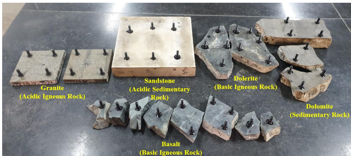
Figure 3-27. Sample for BBS test by considering different aggregate types
