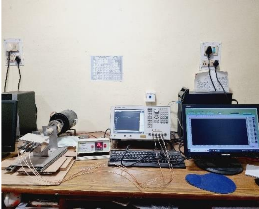
Figure 2.6 Experimental setup to measure temperature dependent dielectric properties using Keysight impedance analyzer.
