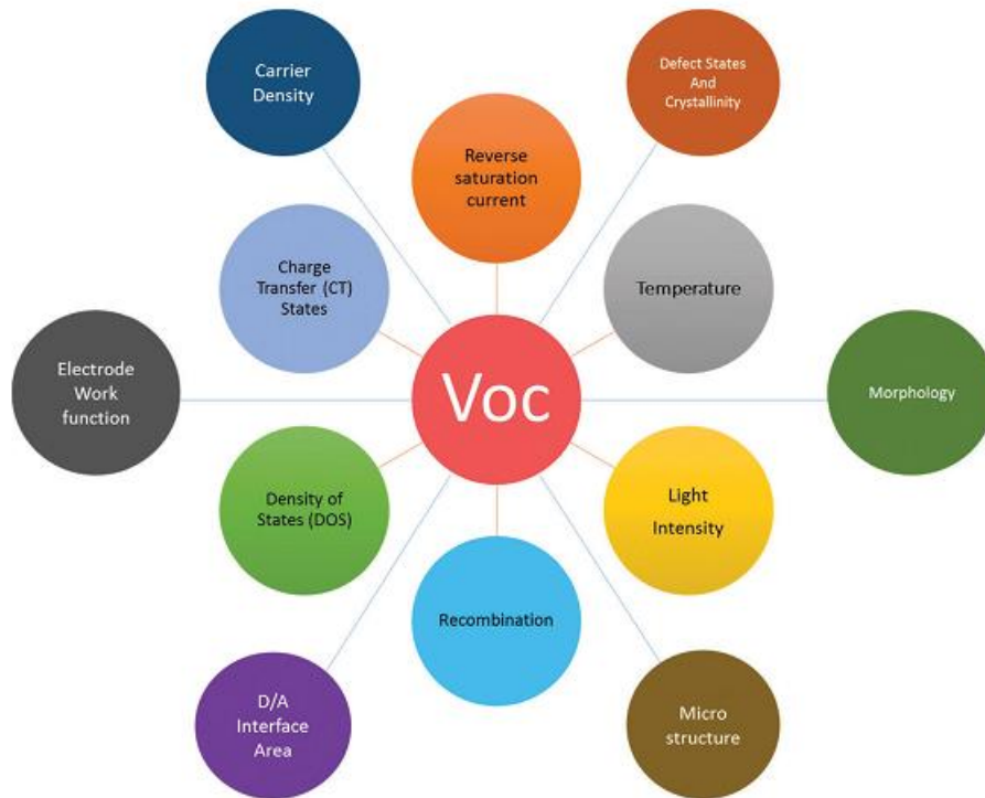
Figure 1.12: Factors influencing the open-circuit voltage in OPV [40].
