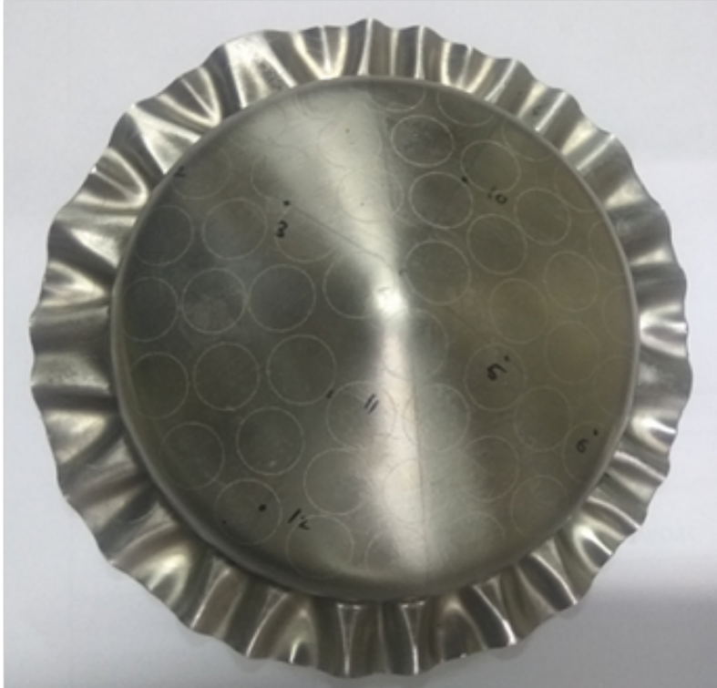
Figure 5.3: Component formed by conventional deep drawing
