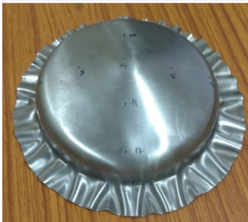
Figure 5.4: Component formed by rubber assisted deep drawing
