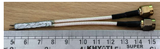
Figure 3.9: Semi-rigid differential probe used for impedance measurement
