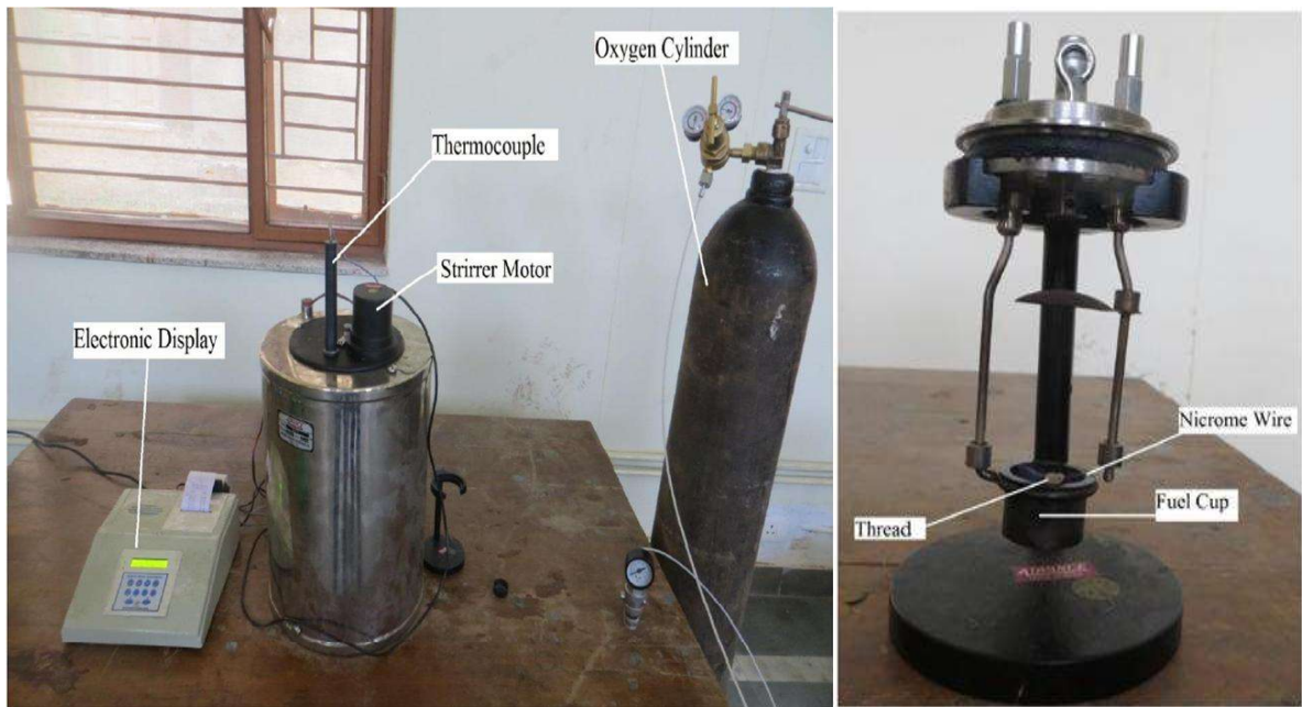
Figure 3.16: Bomb calorimeter and bomb with carrier
